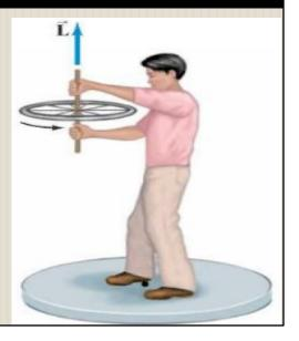
Consider the system of turntable, person, and wheel. The total angular momentum before is **L** upward. Afterward, the total angular momentum must be the same. If the wheel is upside down, its angular momentum is **–L** so the angular momentum of the person must be **+2L**. So the person rotates in the direction the wheel was initially spinning.
